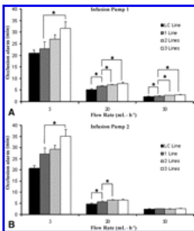
**Figure 1.** Occlusion alarm times (min) of 2 different infusion pump systems (A, B) of the same model at flow rates of 5, 20, and 50 mL/h with 1 (1 Line), 2 (2 Lines), 3 infusion lines (3 Lines) and with a low compliance (LC Line) infusion line. Values are given as means  $\pm$  sd. \*Indicates statistical significance ( $P < 0.05$ ) compared to occlusion alarm time with 1 infusion line.
